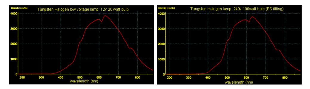
You can see that the spectra for both bulbs are essentially identical- this is simply the emission spectrum from white-hot tungsten. The curve tapers quite smoothly into the UVA range but there appears to be very little below 400nm. Zooming in to the UV range of the spectrogram clarifies the situation: there is no detectable UVB (280 – 320nm) from either bulb.
